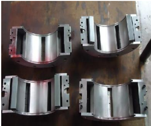
Fig. 2. Journal bearing (segmental type)
