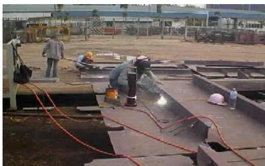
Fig. 3.2.1 Ship's Block Fabrication Process
