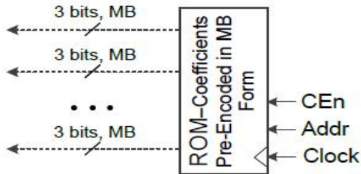
Fig.4 the ROM of Pre-Encoded multipliers with standard coefficients in MB form.
