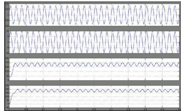
Fig. 13. results of the dc-ac inverter for the proposed transformerless grid-connected power converter under the steady state. (a) Utility voltage. (b) Output current of the dc-ac inverter. (c) Capacitor voltage Vdc2 . (d) Capacitor voltage Vdc3 .
