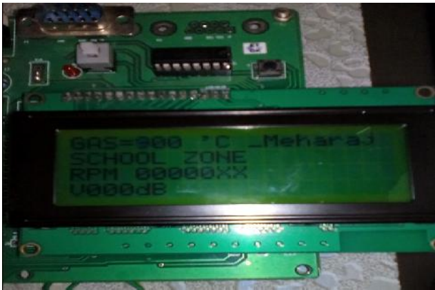
Fig. 13(a) Signal unit sensed SCHOOL ZONE
