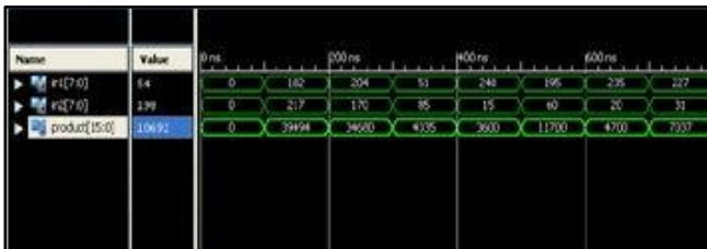
Fig. 9: Compressor Based Vedic Multiplier Wave Forms
