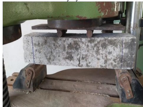
Fig. 8. d) Bending tensile strength two-point test reinforced concrete with Glassfibers. This also demonstrated a strong correlation between the model of bending tensile strength dependence and the fiber quantity. The R2 value was determined to be 88.8% for fiber reinforced concrete with Steel fibers, and 99.3% for fiber reinforced concrete with Glassfibers.
