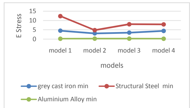
Fig no. 4.7 Graph Showing Minimum Equivalent stress (Mpa) differences for the Materials Grey cast iron, steel, aluminium alloy
