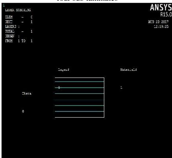
Fig-1 Modeled laminated composite beam with four sub laminates
